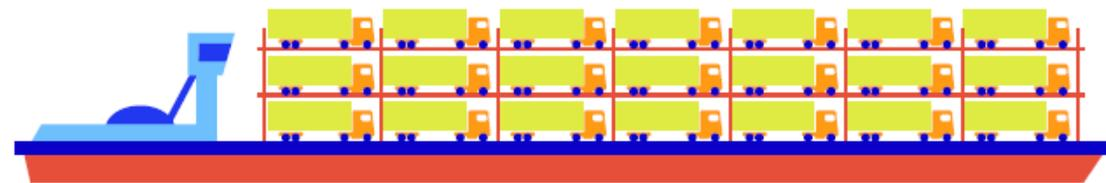
1 AUTOMOTEUR FLUVIAL DE 4400 TONNES TOUTES LES 1/2H ÉQUIVAUT AU PASSAGE D'UN CAMION (25 T) TOUTES LES 5 SECONDES
